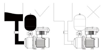
(4) As shown in the figure, do not cover the pump with fabric, wrapping paper, etc. to keep warm, otherwise the motor and inverter cannot dissipate heat and may cause fire.
